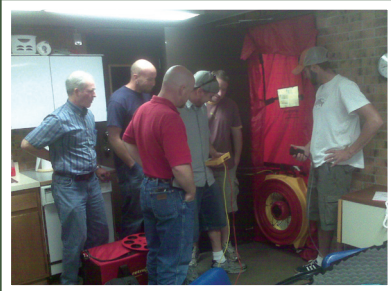
Instructors Deacon Taylor and Ed Hegwood with student interns conducting blower door testing at The Learning Source.
